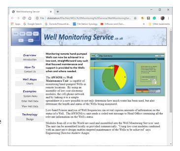
Low-band Fourier analysis of Well frequencies can reveal copious amounts of information on the status of a Well. The AWSOM<sup>(TM)</sup> unit sends a coded text message to Head Office containing all the relevant information on the Well's status.
