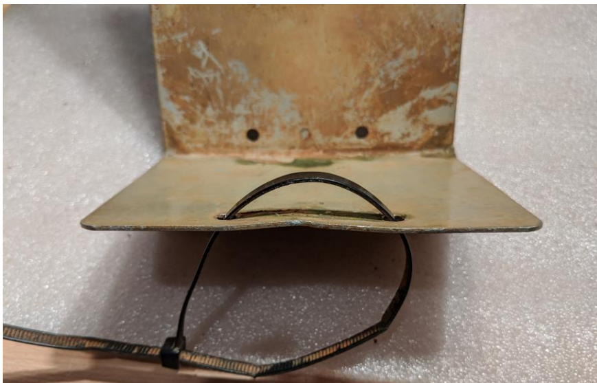
Figure 10: Vertical Plate Warping
