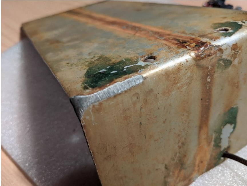
Figure 9: Base Plate Corner Stress
