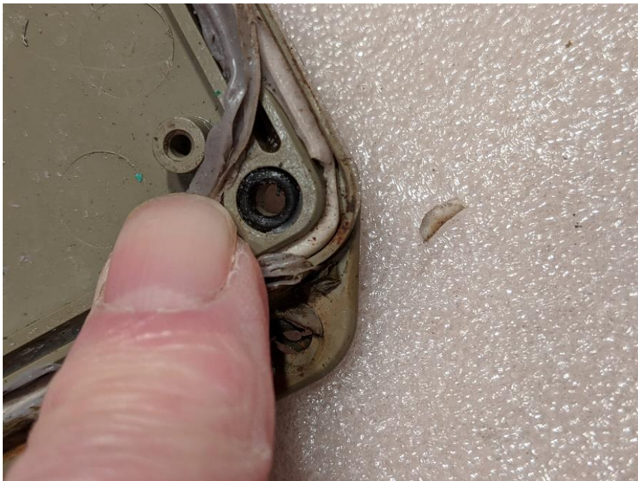
Figure 5: Unit #3888 Housing Base's Distressed White Rubber Seal
