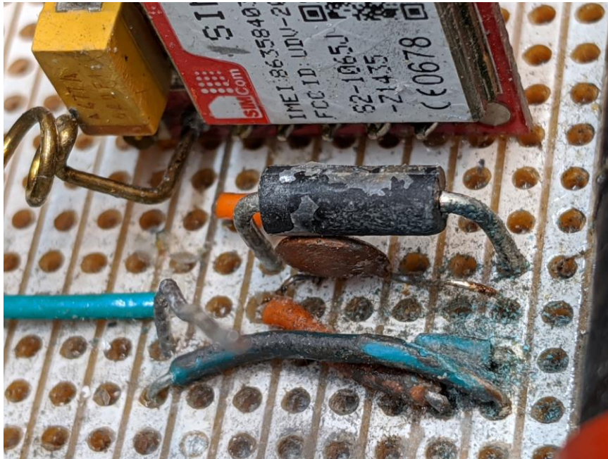
Figure 16: Chipped Conformal Coating on Zener
